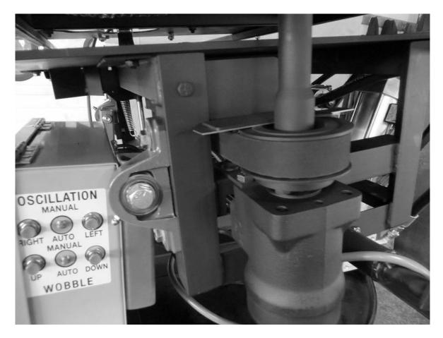
Install the bracket using a shim between the top of the pulley wheel and bracket. A machinist ruler is shown but you can use a piece of cardboard from a shotgun shell box (.050"). The washer and nut need to go on the back side so that the washer covers the slot on the deflector. Once the bolt is secured remove the shim.
