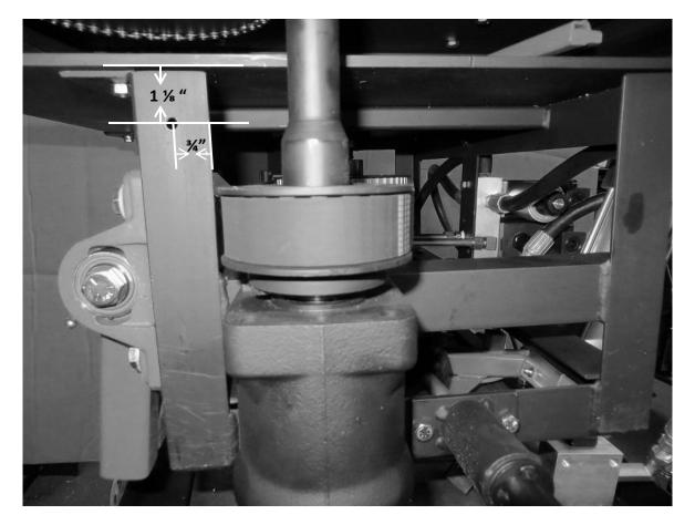
To mount the debris deflector (PT 9050) prick punch a hole  $1 \frac{1}{8}$  " down from the bottom of the throw plate and  $\frac{3}{4}$ " from the right side of the angle iron. Drill pilot hole using a  $\frac{1}{8}$ " drill bit; complete the hole with a  $\frac{1}{4}$ " drill bit.
