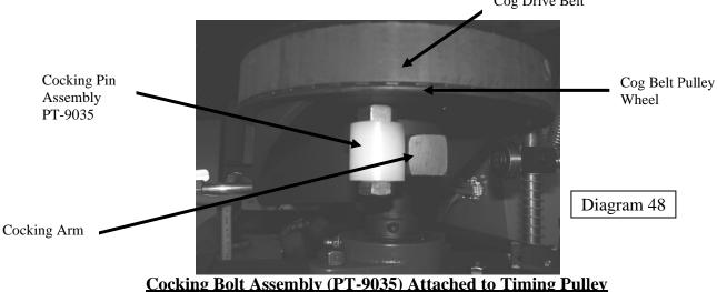
IMPORTANT: Do not tighten the bolt against the nut because it will compress the bumper.
