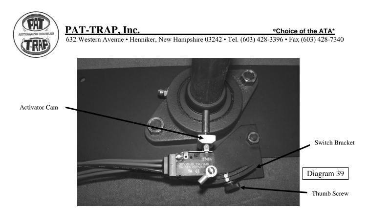
Top View of #2 & #3 Switch Bracket shown on Activator Cam
