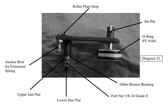
If an adjustment is necessary, then the roller plate stop will have to be turned until the roller plate stops at the given measurement.
