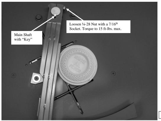
5. Pry downwards against the underside of the top plate to install the new throw arm.
