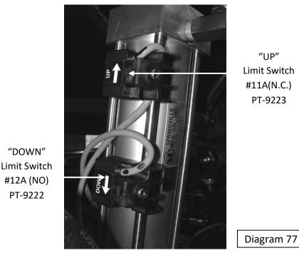
Limit Switches on the PAT-TRAP<sup>®</sup> Wobble Hydraulic Cylinder
