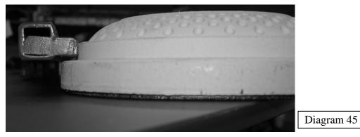
Setting Correct Target Clearance for Throw Arm with a Target
