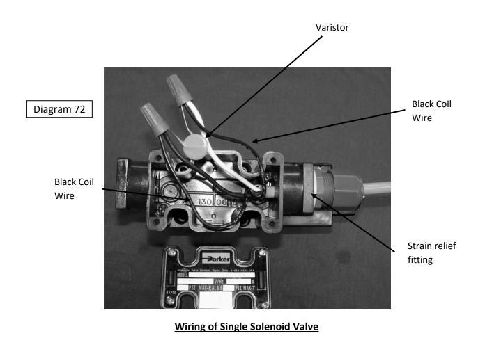
Connect one of the valve's black coil wires to each of the black and white wires entering the strain relief fitting along with a leg from the Varistor as shown above.
