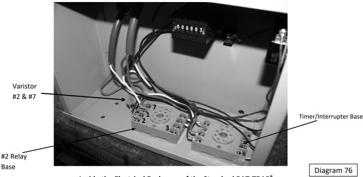
Inside the Electrical Enclosure of the Standard PAT-TRAP<sup>®</sup>
