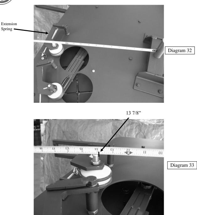
Singles Roller Plate measurement is 13 7/8" from face of Kingpin Shaft to inside face of the Single Roller Wheel bolt.
