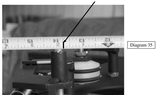
Doubles Roller Plate measurement is 13 <sup>3</sup>/<sub>4</sub>" from the face of the Kingpin Shaft to the inside face of the Doubles Roller Wheel bolt.
