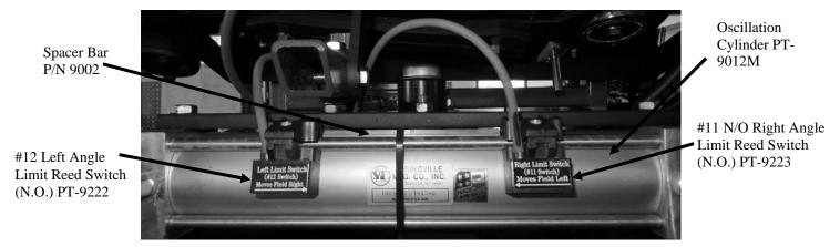
Pat-Trap® #12 & #11 Limit Reed Switches on Oscillation Cylinder
