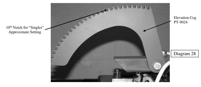
**Elevation Cog on Front of PAT-TRAP®**
