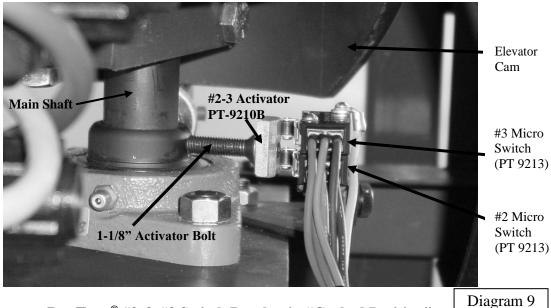
Pat-Trap<sup>®</sup> #2 & #3 Switch Bracket in "Cocked Position"
