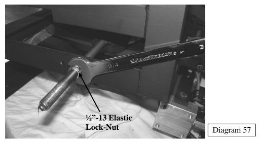
Adjusting Elastic Lock Nut with 3/4" Wrench
