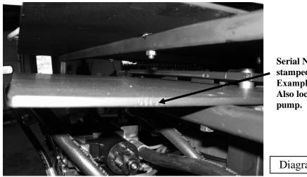
Serial Number is stamped here. Example: "G4190" Also located on
