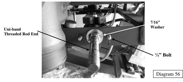
**Removing Main Spring Standoff Collar Sleeve**
