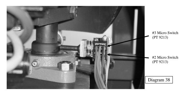
Side View of #2 & #3 Switch Bracket shown on Activator Cam
