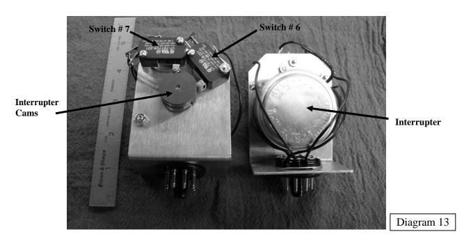
Front and Rear Views of Interrupter (PT-9216) for PAT-TRAP®
