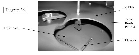
**Installation of New Target Brush**
