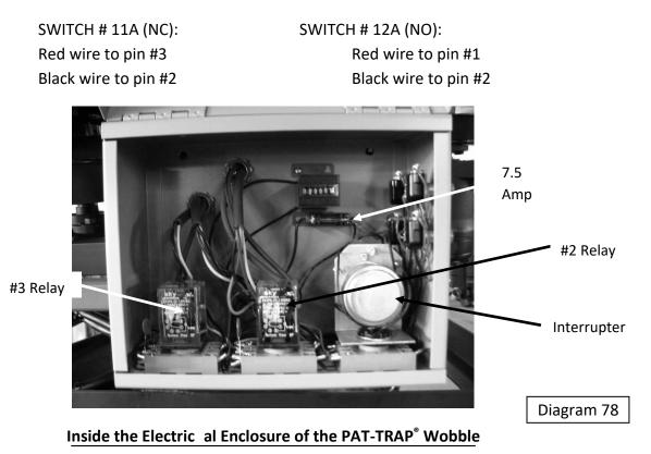
5. After replacing the appropriate Up or Down Wobble limit switch, close and secure the rear cover of the electrical enclosure. Connect the PAT-TRAP<sup>®</sup> back to its power source and resume operation.
