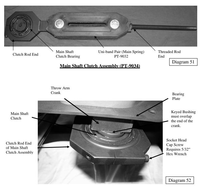
Clutch Rod End of Main Shaft Clutch Assembly
