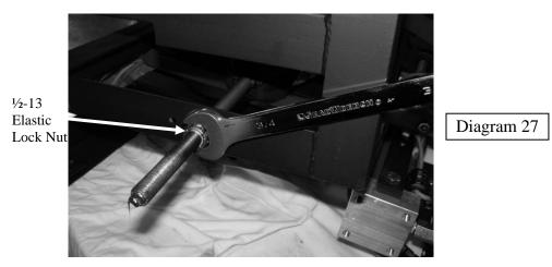
Adjusting Elastic Lock Nut with 3/4" Wrench
