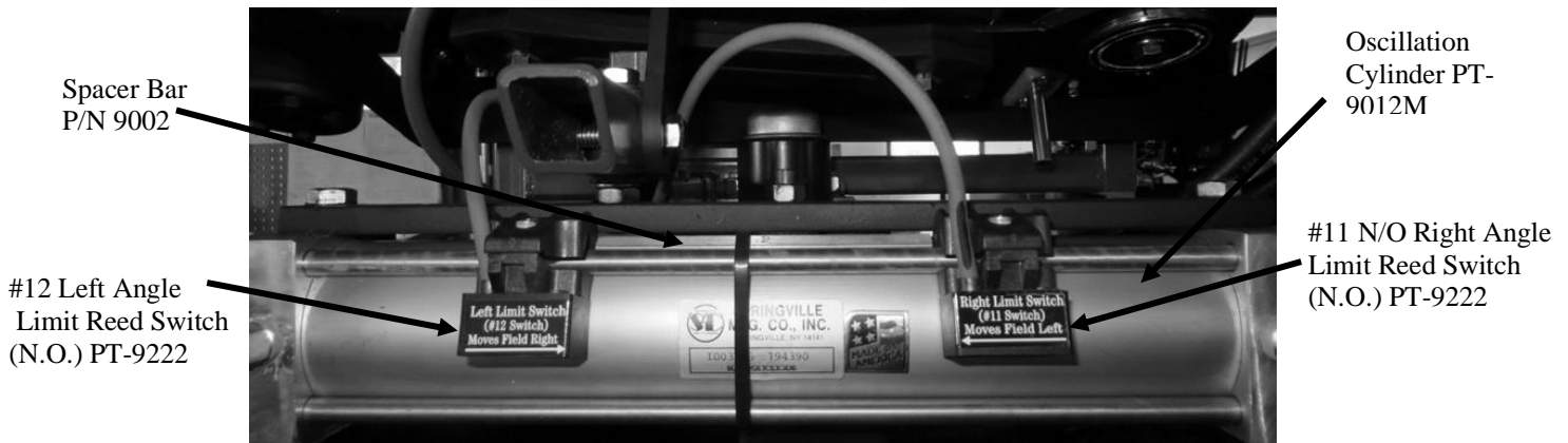
Pat-Trap® #12 & #11 Limit Reed Switches on Oscillation Cylinder
